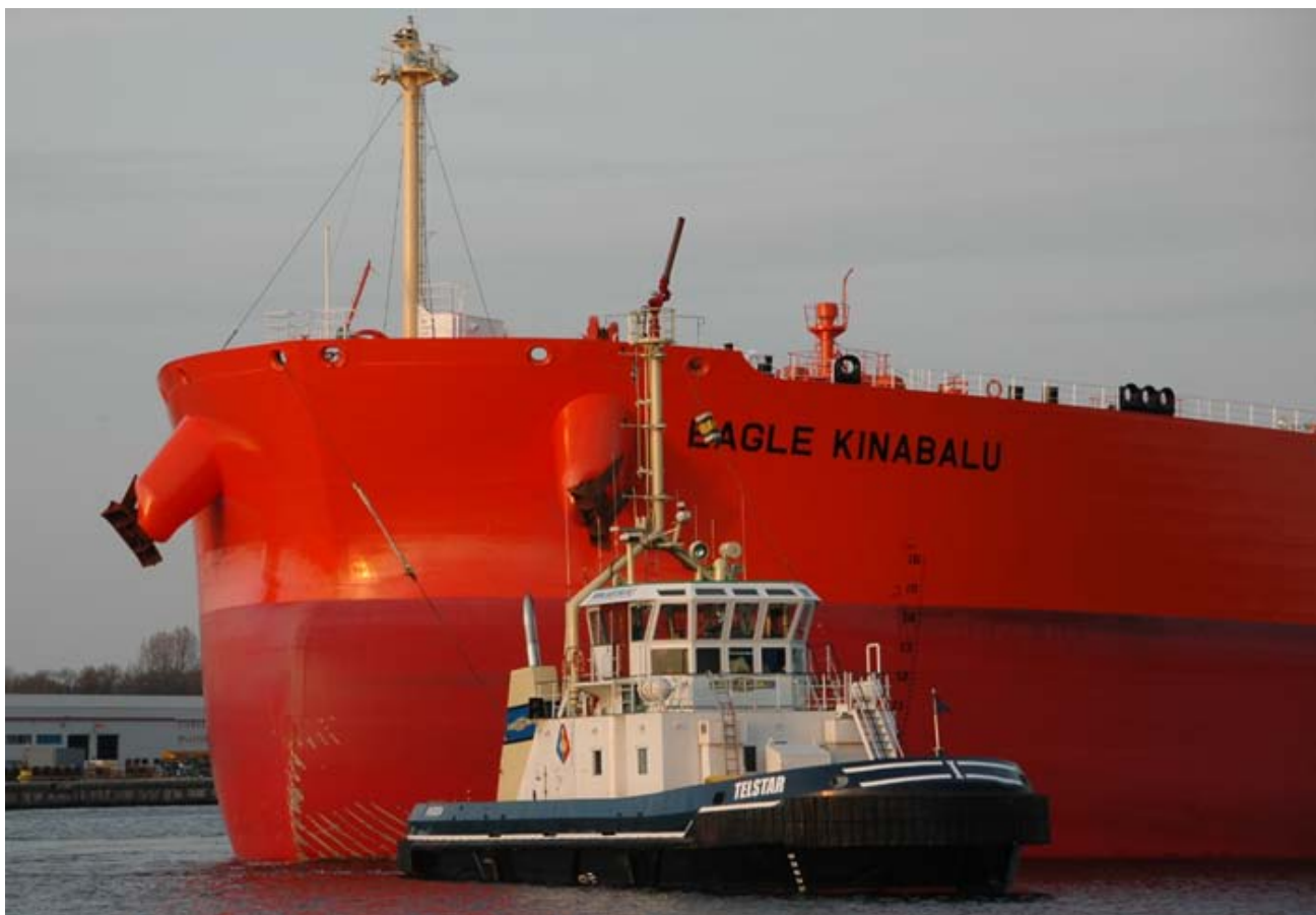
Iskes TELSTAR seen with the brandnew (2011 delivered) AET tanker EAGLE KINABALU (107.481 DWT) in IJmuiden, the crude oil tanker is powered by a MAN-B&W engine built by Mitsui Engineering & Shipbuilding C Ltd – Japan with an output of 18,436 hp at 105 rpm for a top speed of 16 knots Photo : Joop Marechal ©
