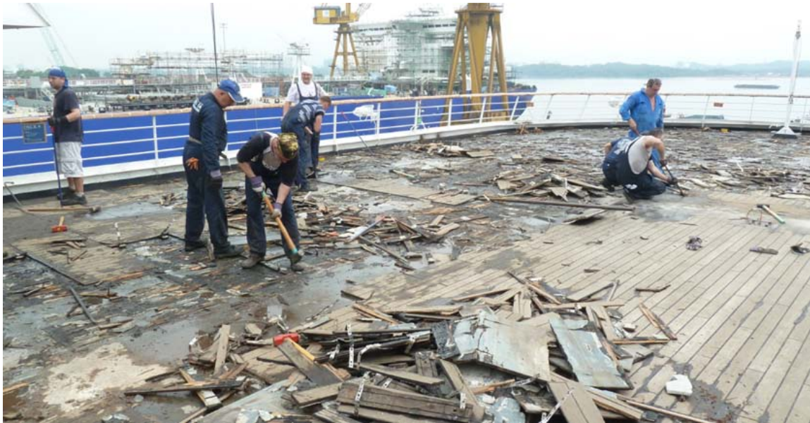
All the teak wood at the Lido deck will be removed and is replaced by a new « teak » polymer
