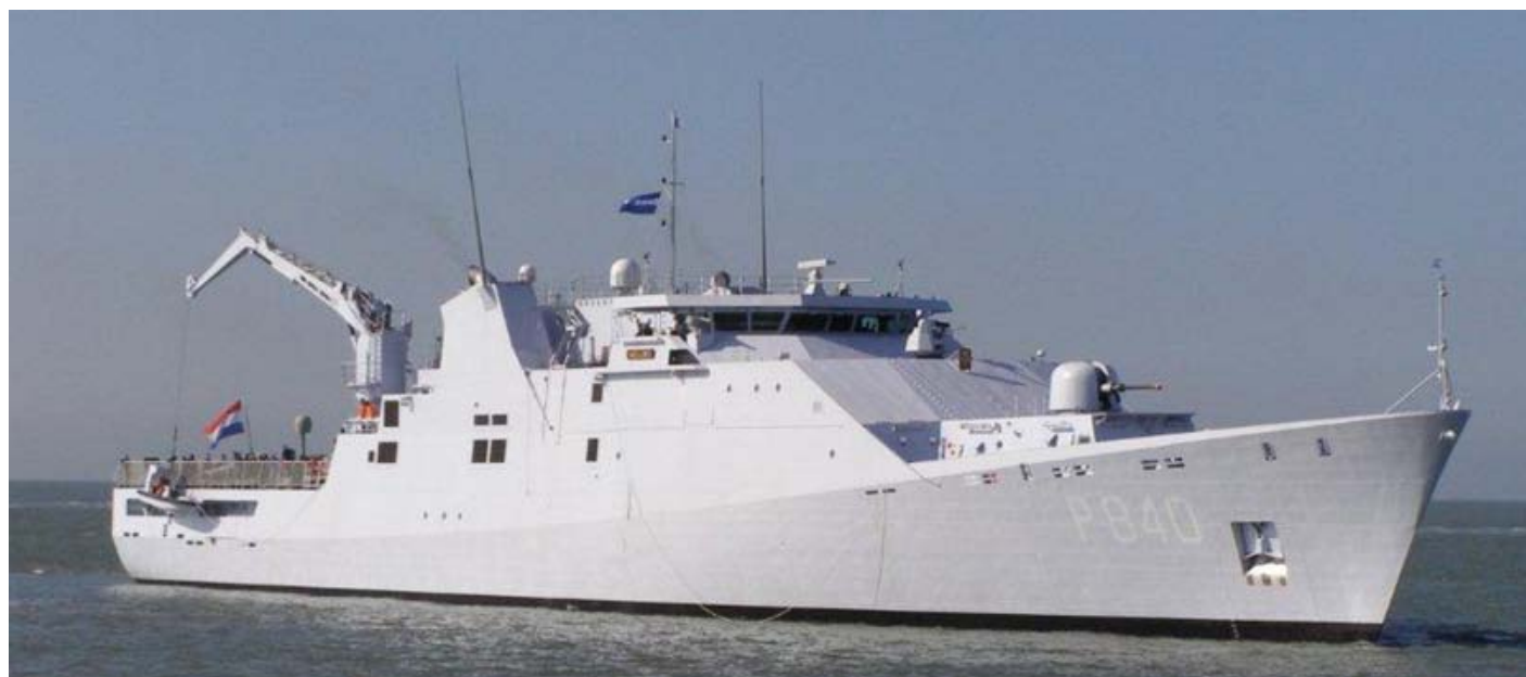
The P 840 HOLLAND commenced yard trials last Monday at the Westerscheldt River, as can be seen the mainmast with the radars and other sensors is not installed yet, instead a temporarily mast is installed for the navigation lights
