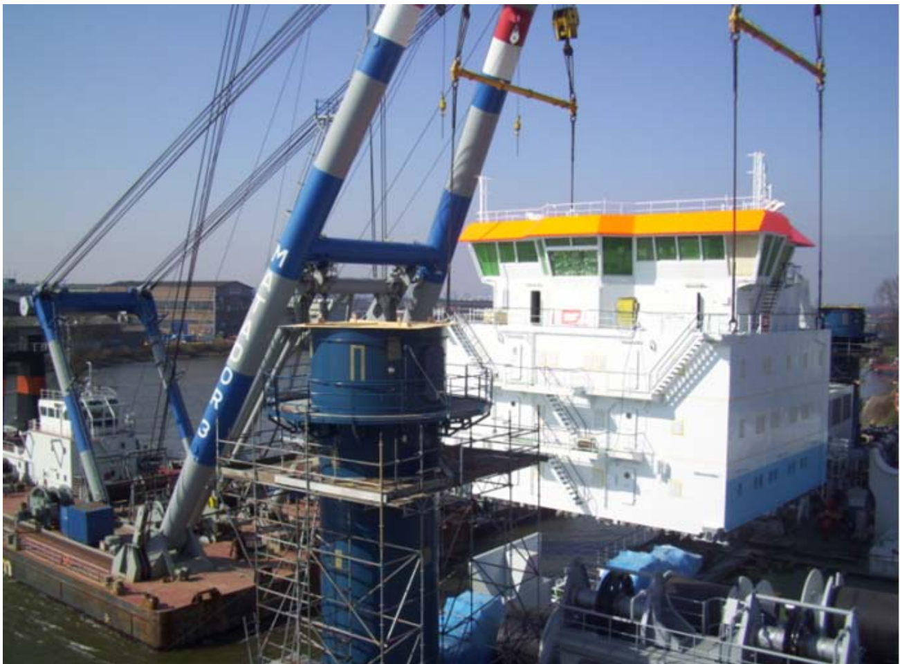
The sheerlegs MATADOR 3 seen lifting the accommodation module onboard the ATHENA in Kinderdijk (Holland) Photo : Reinier Roest (c)
