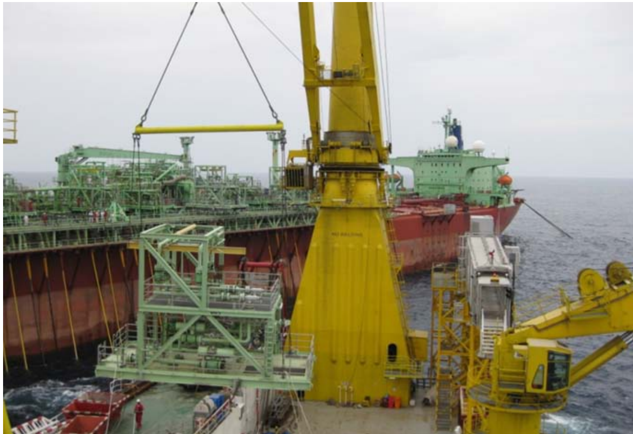
The JASCON 34 successfully installed 3 flowline modules onto the FPSO SENDJE BERG in the Okwori field, Nigeria. Photo : Capt. Peter Lankester (c)
