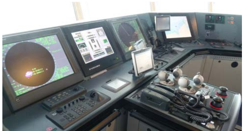
Top : The front manoeuvring panel and left seen the modern engine controls, below one of the two chairs at the aft panel, with built in the controls and ofcourse a coffee/tea cup holder
