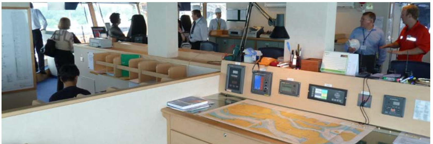
The spacious wheelhouse with in front the chart table and navigation instruments
