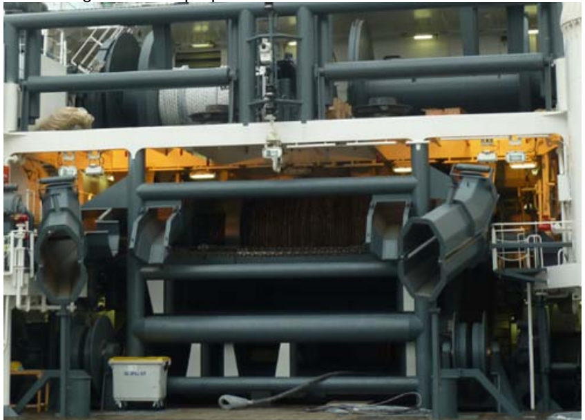
The AHTS is equipped with a 400 tons (pull) (500 tons-stall) winch, and several storage reels as can be seen above
