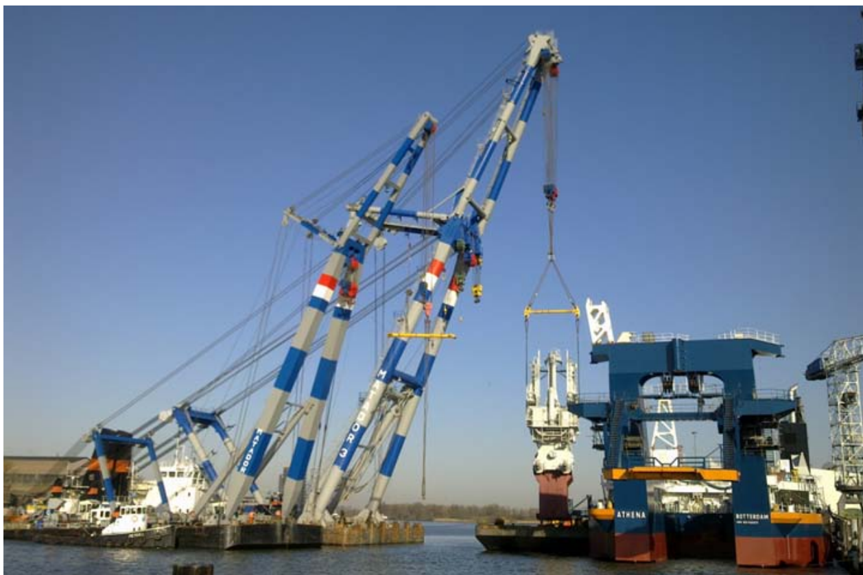
Above seen the sheerlegs Matador 3 ready to install the spudcarrier into the recently launched CSD Athena of Van Oord. The Matador 3 was assisted by the Matador to bring the spudcarrier into an upward position. The Matador was assisted by Pieter L. Photo : Wim Ooms ©
