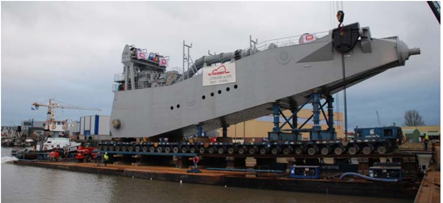
The IHC-Beaver built 1460 ton (in weight) cutter ladder for the CSD ATHENA was driven onboard a barge in Sliedrecht by SARENS – Photo : Jan van Heteren ©
