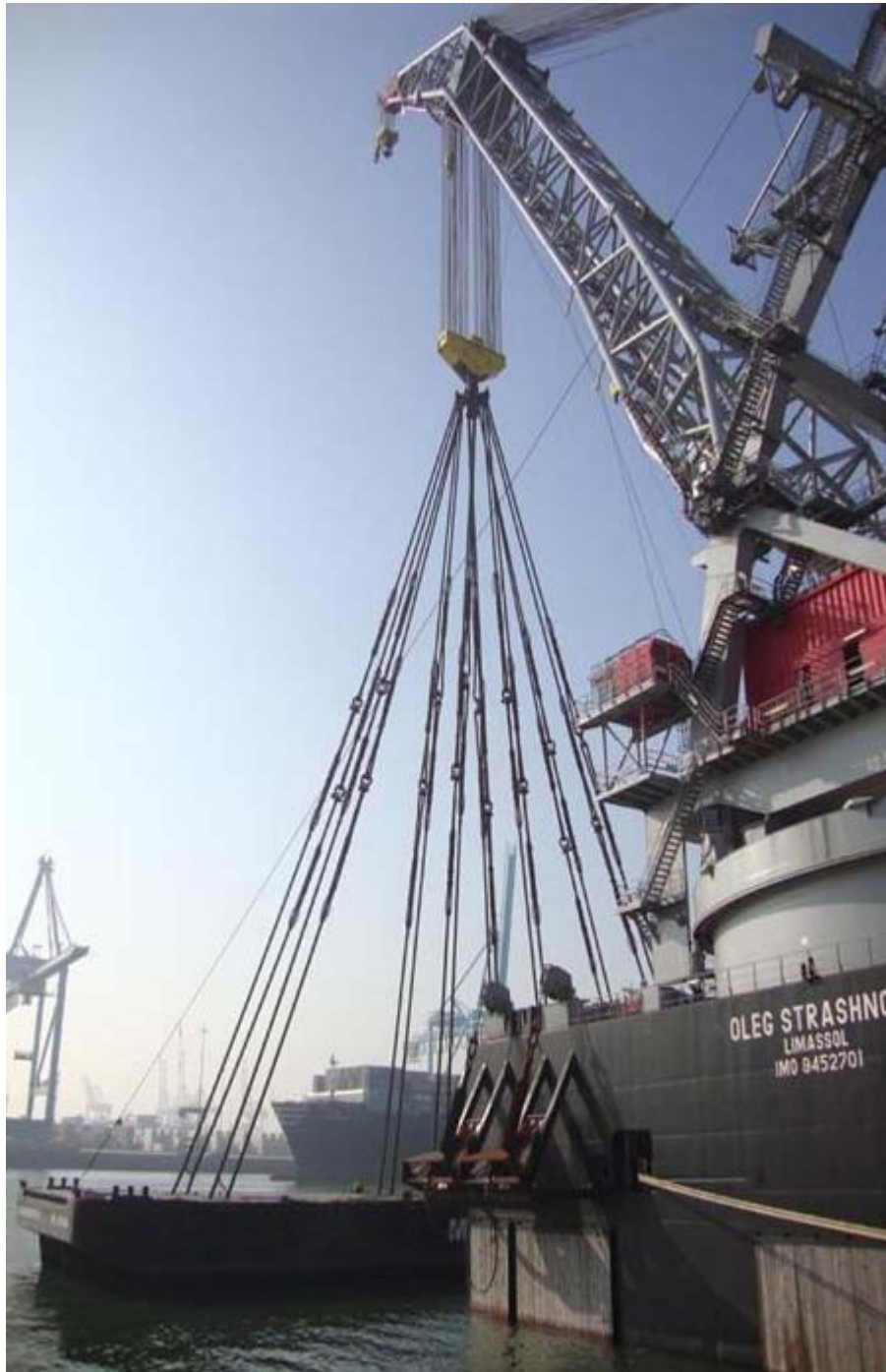
The Oleg Strashnov prepared for 5500T test lift by Muller Dordrecht and Franklin Offshore Photo : Jerry Bakx - Franklin Offshore Europe - www.franklin.com.sg ©
