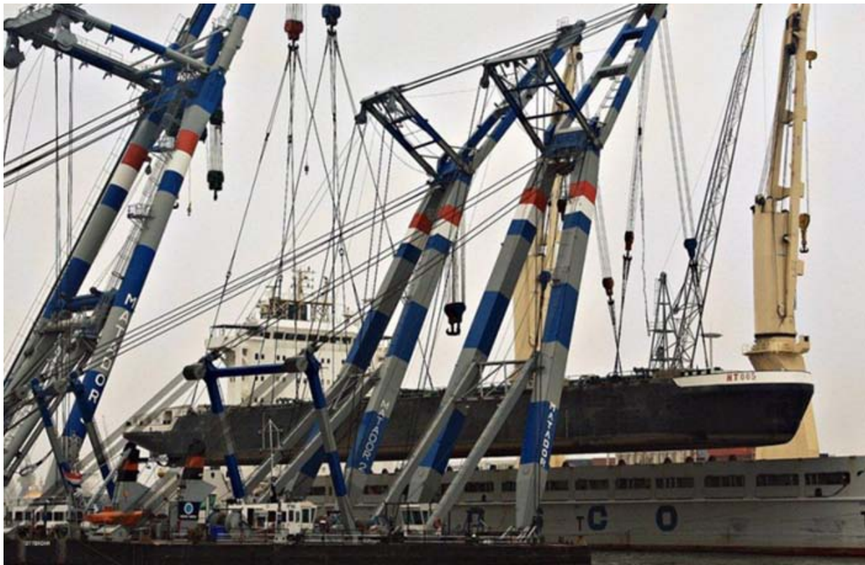
Several MATADOR shearlegs seen in Rotterdam-Waalhaven lifting a newbuilding hull Photo : via Ruud Breur
