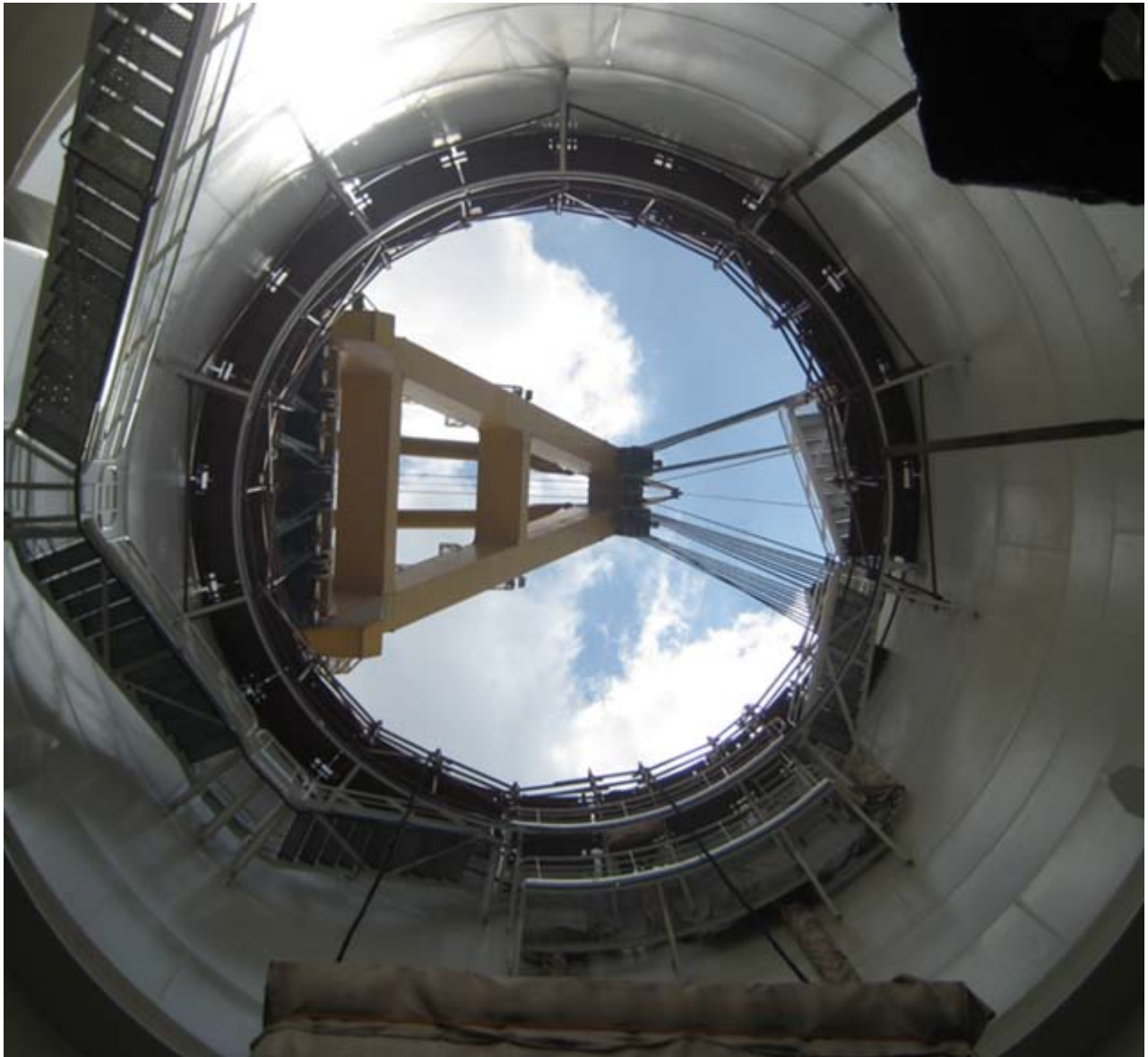
Photo made from the inside of the pedestal of the 5000 tons HUISMAN crane onboard the BOREALIS just prior the installation of the 1124 tons Slewing unit by the sheerlegs ASIAN HERCULES II
