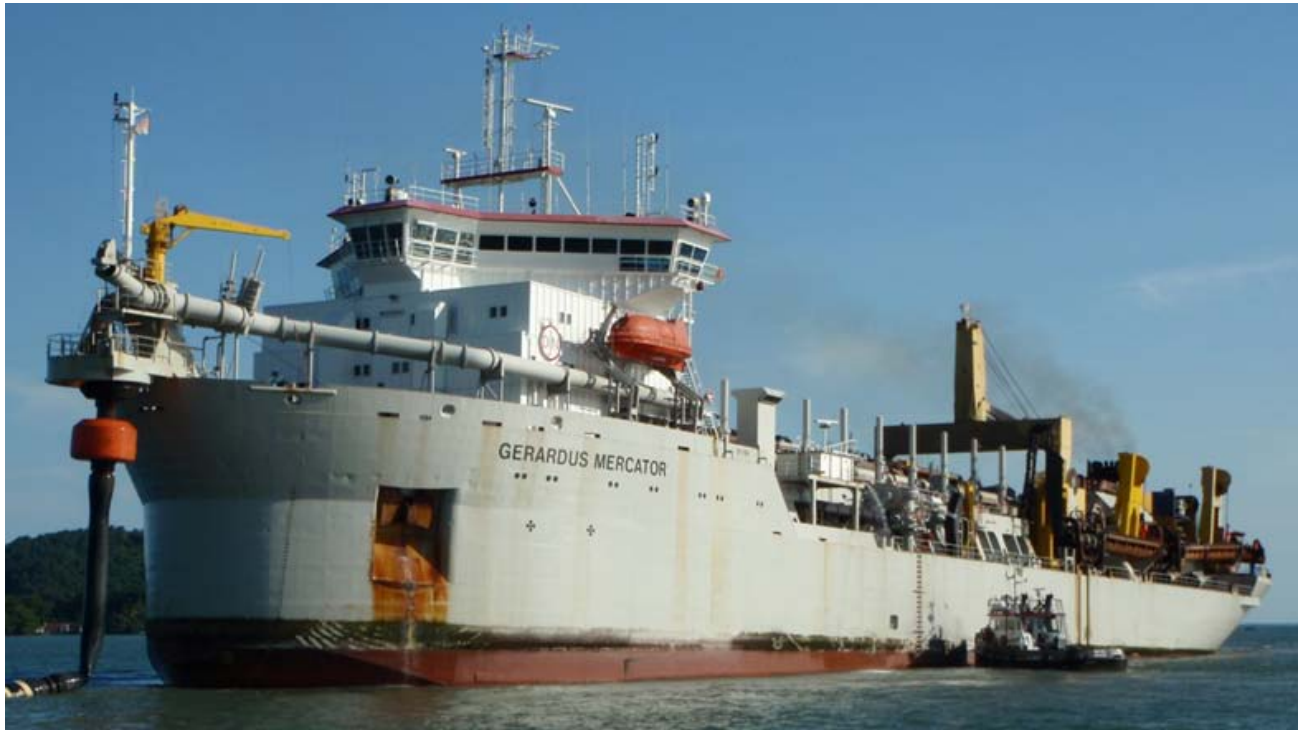
The TSHD GERARDUS MERCATOR seen coupled to the CSD Hondius in the Port of Itaquai (Brasil). Here Jan de Nul is working on the construction of the new (Naval) base for Submarines
