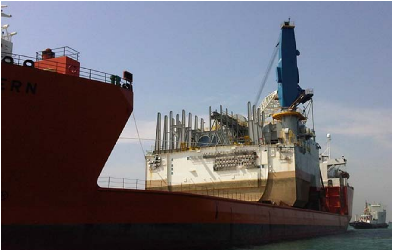
Dockwise TERN loaded with sternblock section of Noble Leo Segerius seen in Singapore the sternblock will be transported by the TERN to the BrasFELS yard in Brazil - Photo : Jan Wolter Oosterhuis ©
