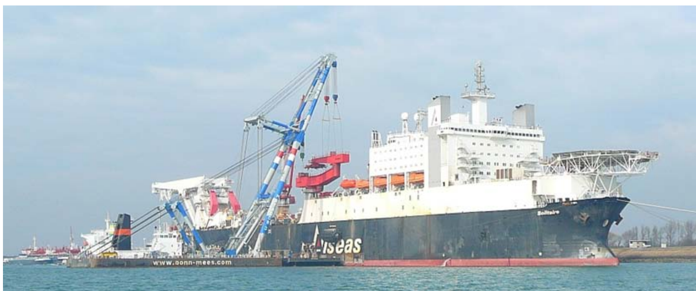
Above the Solitaire and the Matador 3 seen in the Caland canal Rotterdam. Matador 3 is lifting Solitaire's pipe transfer crane due to a maintenance job. Photo : Arjen Perdok ©
