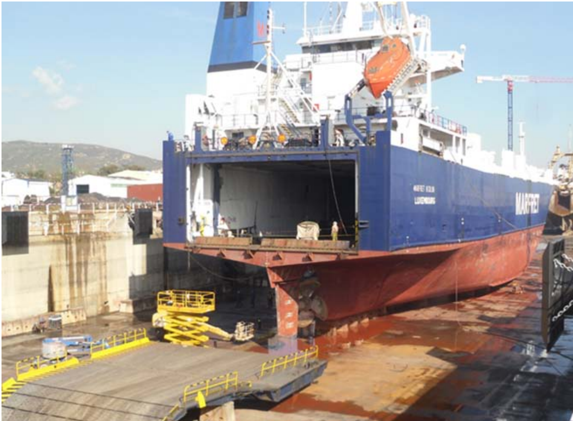
The RO - RO vessel " MARFRET NIOLON " belonging Marfret Marsella, France, under dry docking works and large Stern Ramp repairs at CERNAVAL Shipyard in Algeciras, Spain. Photo : David North ©
