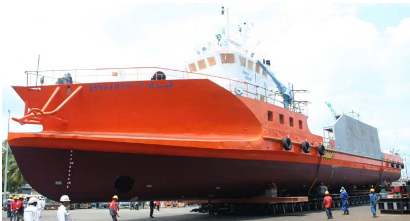
Above seen shifting the Esnaad 810 ( weight 300 Tons ) from fabrication hall to the water front at the Pelican Shipyard in Singapore
