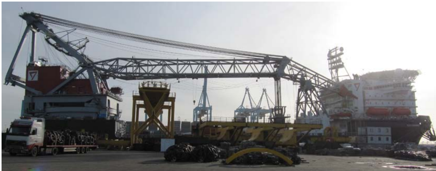
Above seen the Oleg Strashnov during the A-frame lowering test conducted at 3 rd February , at the photo the A-Frame is seen nearly in the lowest position
