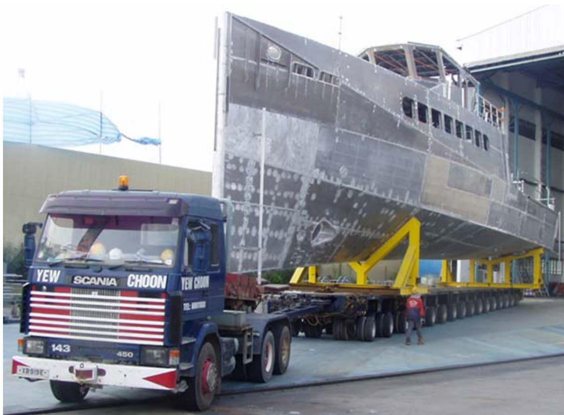
YEW CHOON seen driving a aluminium newbuild hull out at the Damen Singapore shipyard
