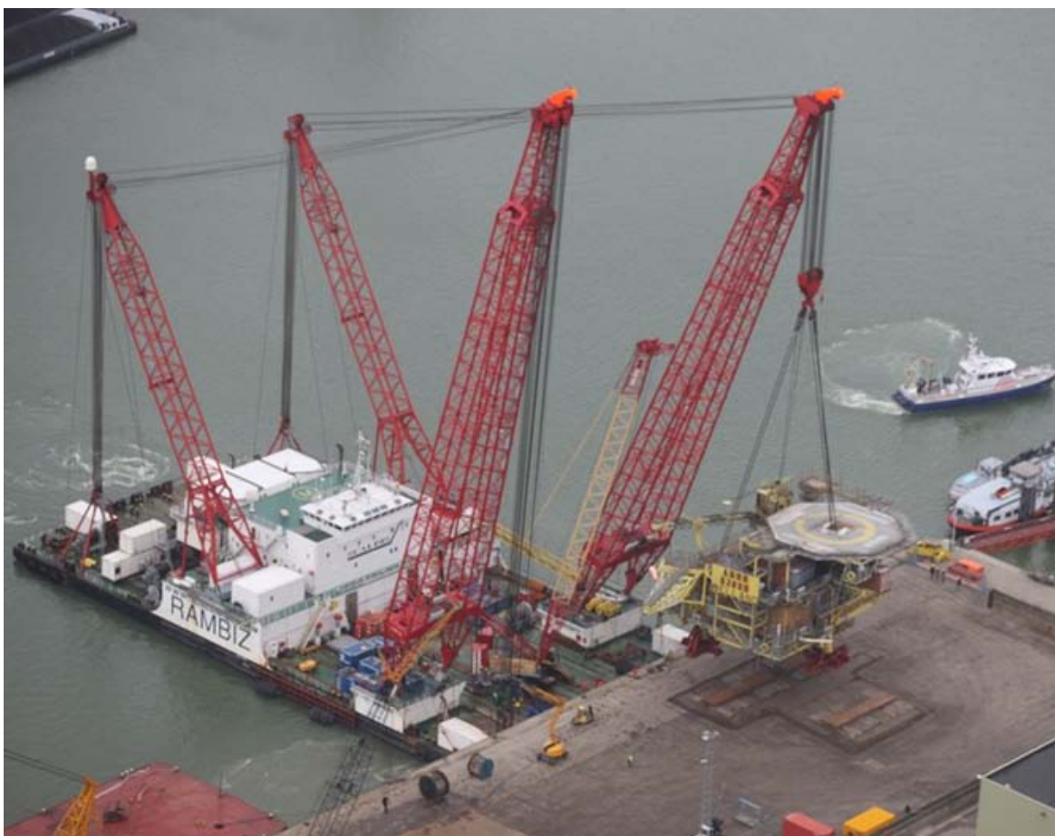
Seen at 24-01-2011 from the sky, HLV " Rambiz " lifted the " Welland " topside from a barge to the shore at the Hoondert yard at Vlissingen. The platform was earlier this week lifted from its jacket at the North Sea.
