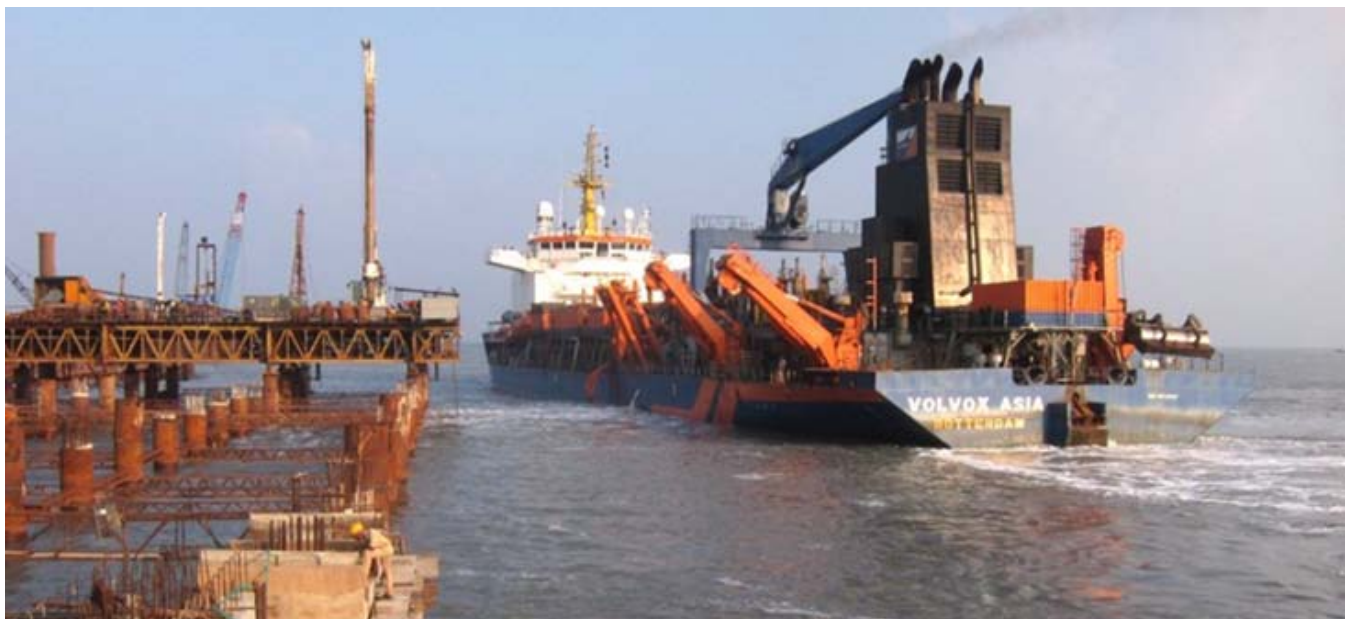
Van Oord's TSHD VOLVOX ASIA seen dredging in front of quaywall under construction in Kattupalli (India)
