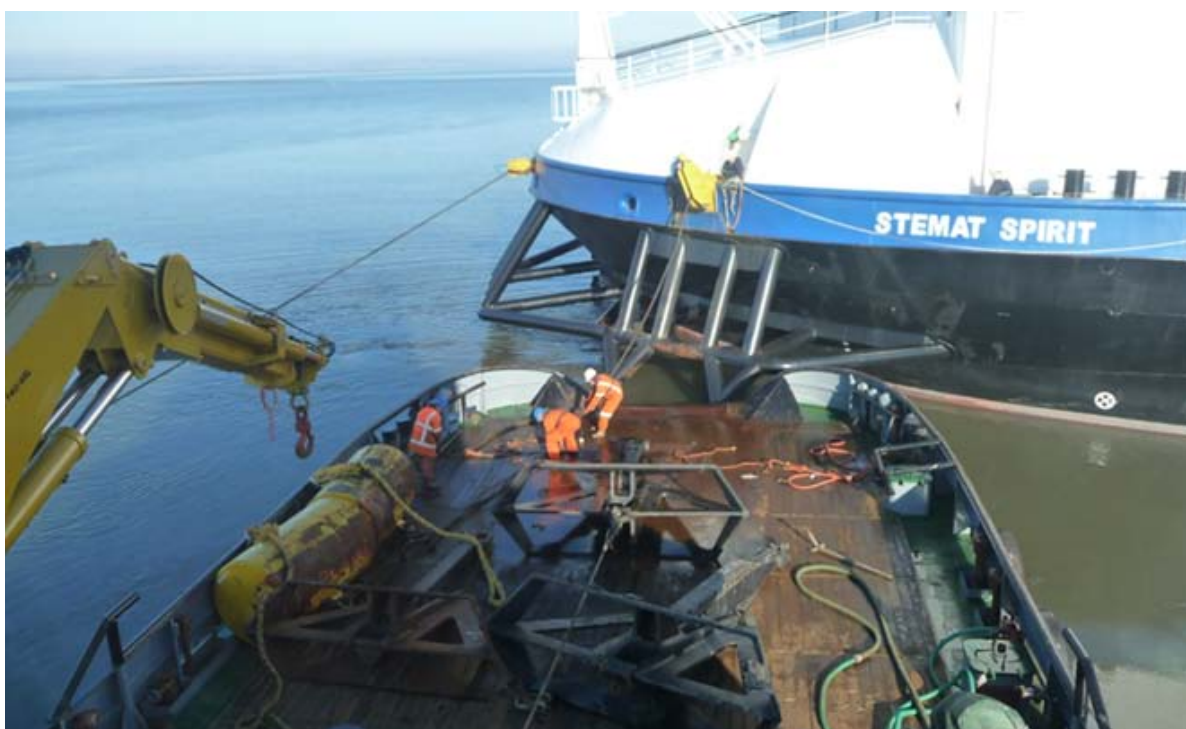
Anchorhandling works ongoing onboard the NEPTUN 9 to deploy the anchors of the STEMAT SPIRIT off Heysham
