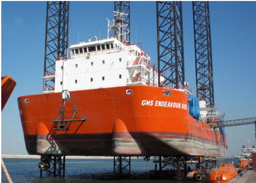
The new GMS Endeavour seen jacked up at the Esnaad base in Musaffah, UAE for thruster installation. The barge will enter her charter later this year on the North Sea for installation of wind turbines at the Sheringham Shoal windfarm off the English east coast. Photo : Bas de Blok ©
