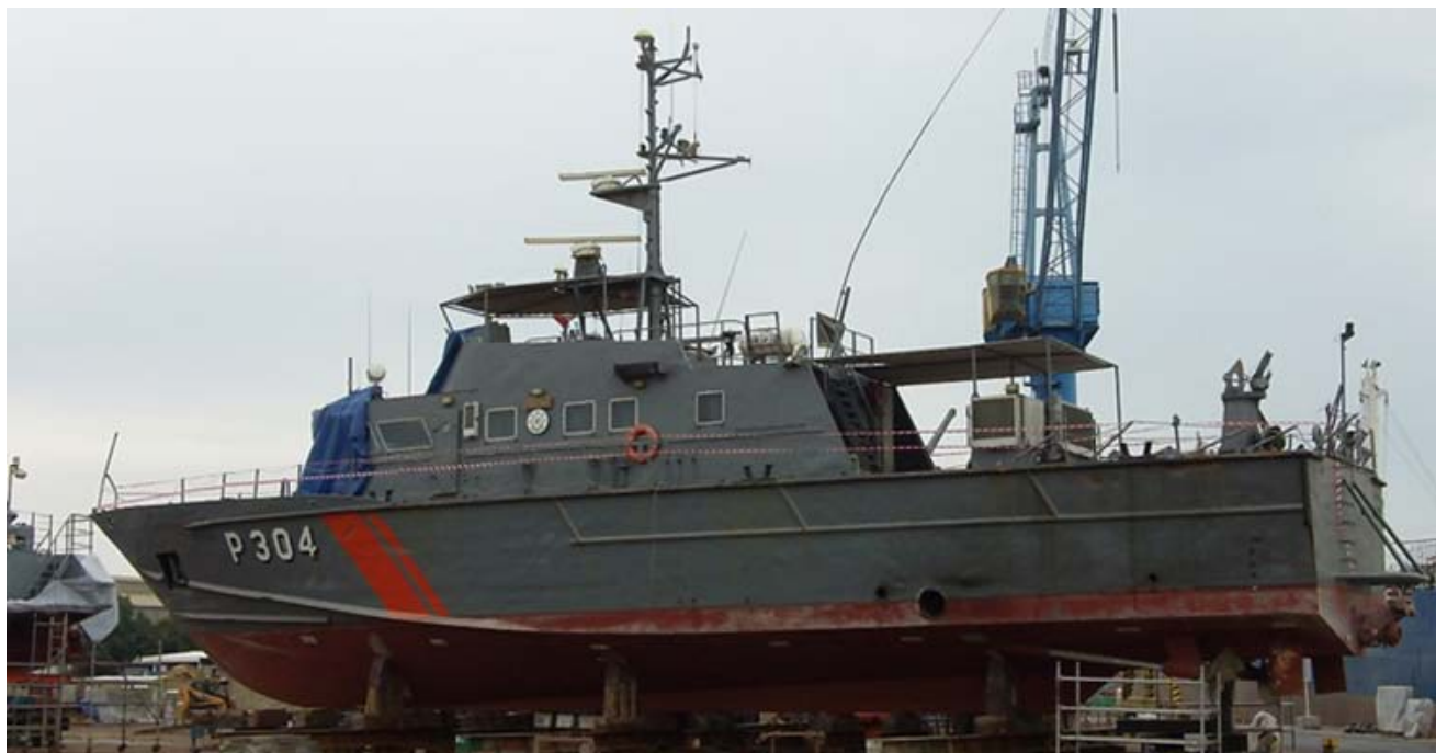
The damaged Kuwait patrol vessel P 304 MOBARK seen at the Heisco shipyard, Kuwait, the 1993 built 32 mtr patrol vessel was involved in a collision incident some weeks ago in Kuwait waters with an Iraqi fishingboat.
