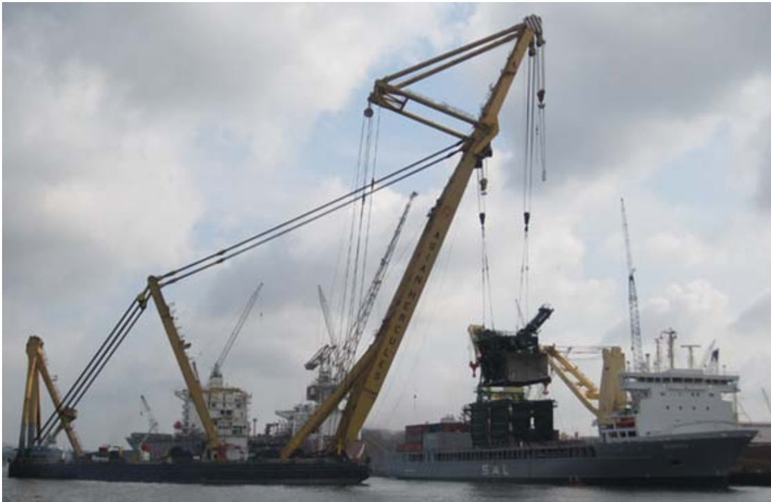
The Sheerlegs ASIAN HERCULES seen offloading the Huisman build 'Stone Dump Unit (SDU)' for DEME. The transport to and installation on the Flintstone was done by the Asian Hercules on 23rd of January Photo's : Ronald Krijgsman ©
