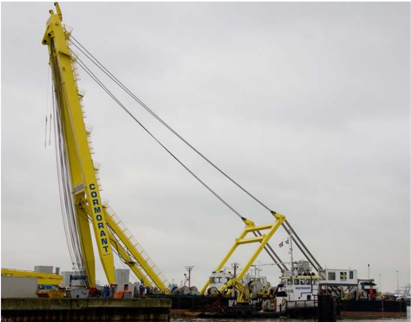
MULTRASHIP's CORMORANT seen with the new A-Frame which was built at VDS in Vlissingen, with the new A-Frame also the lifting capacity of the sheerlegs is increased from 400 to 600 ton
