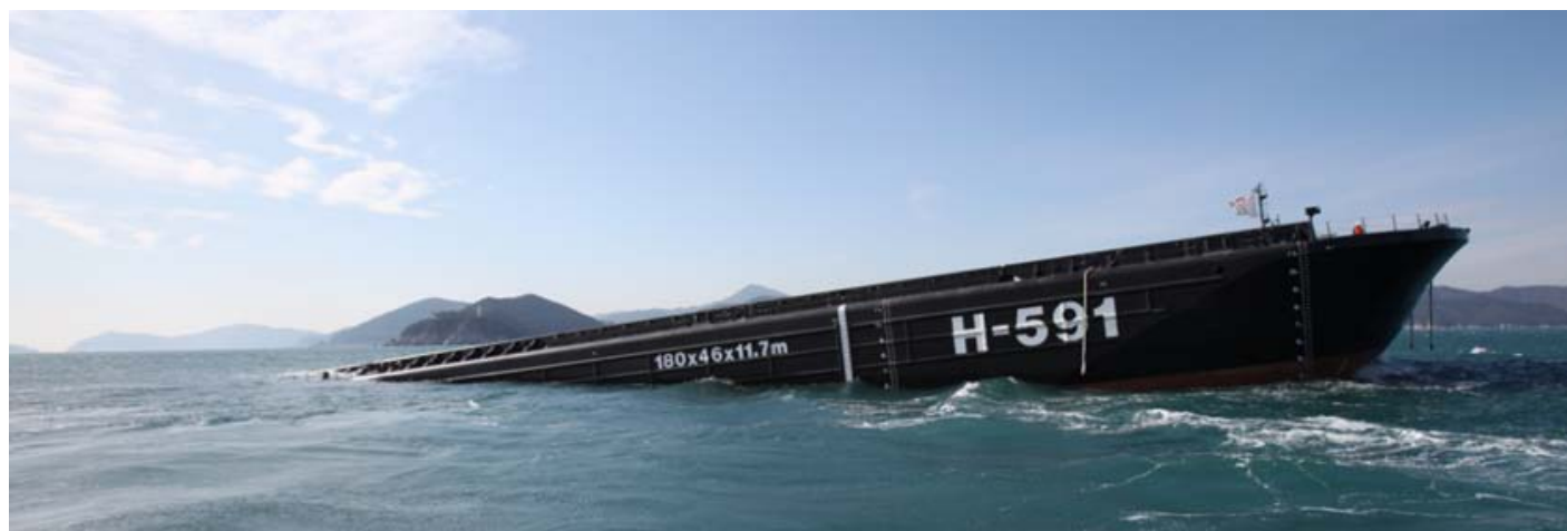
The Heerema Launch barge H591 seen during sea trials submergence tests at Okpo bay South Korea.
