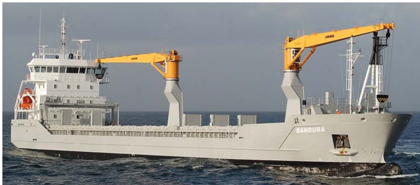
The December 2010 delivered Damen Combifreighter® 8200 118 mtr long BANDURA seen arriving in Willemstad (Curacao), the BANDURA is a multi purpose cargo vessel with a loading capacity of approximately 8.300 tons and equipped with tween decks and two cargo cranes of 40 tons each, on her maiden voyage the vessel has loaded in the Baltic region for a US destination, thereafter via Panama Canal to Asia, the vessel is owned by Noordwijk Ocean Services BV , The Netherlands
