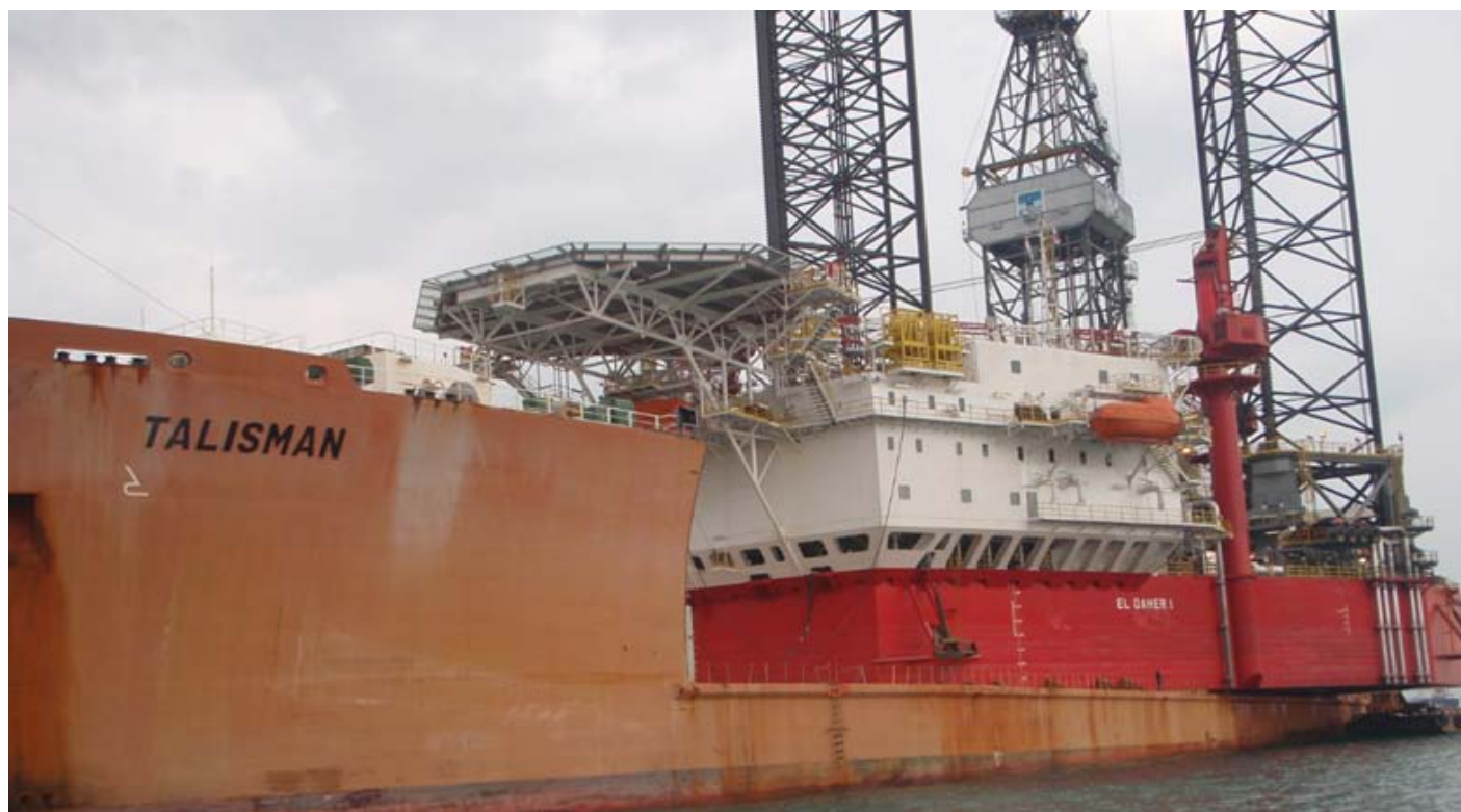
Above seen the loadout of Jack Up rig "El Qaher 1" on the Dockwise Heavy Lift vessel "Talisman" in Singapore, West Jurong Anchorage on 12th January 2011.
