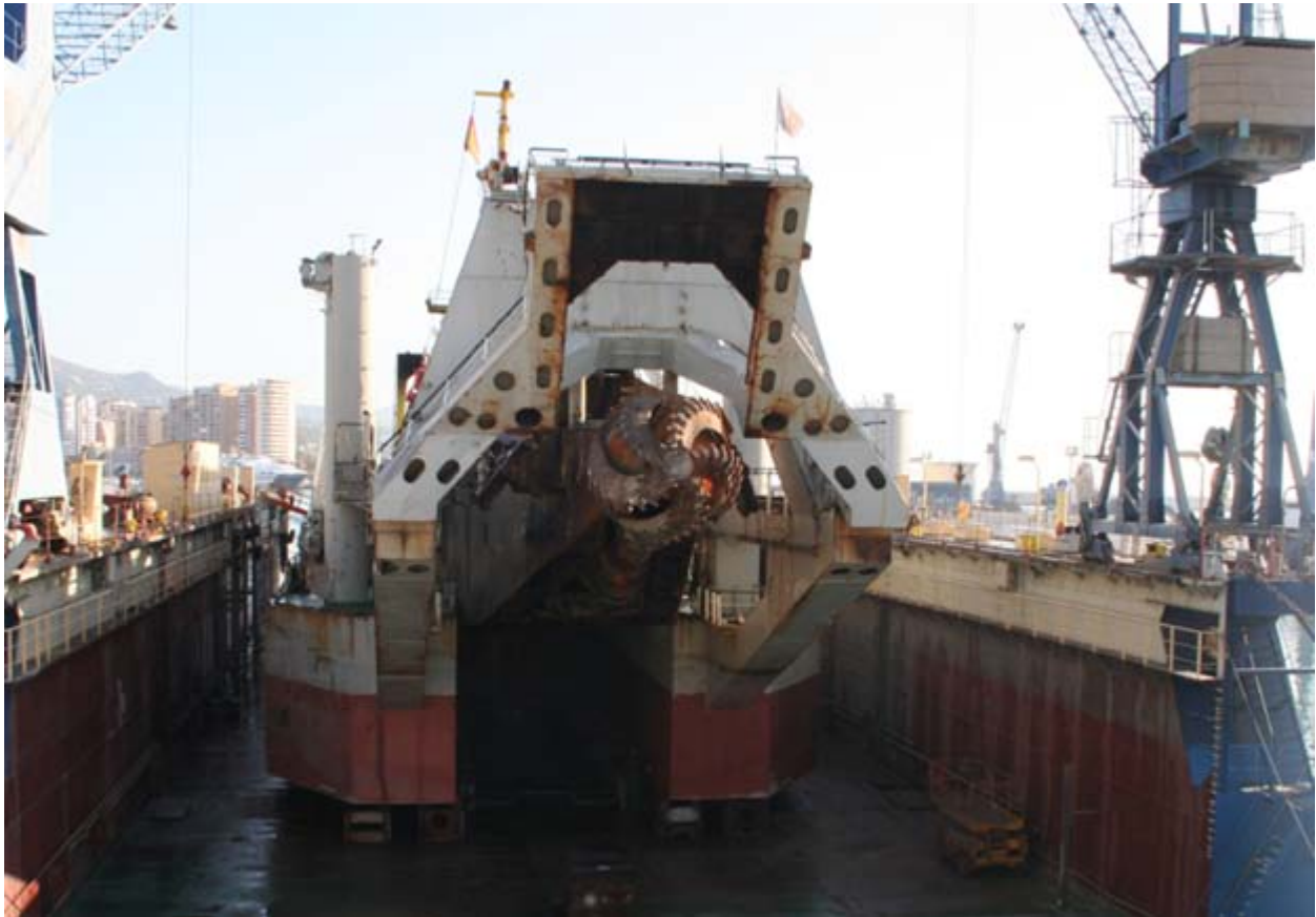
The cutterdredger VESALIUS belonging Jan de Nul, Belgium, under steel bottom damage repairs works at Malaga Shipyard belong CERNAVAL SHIPYARDS GROUP in Spain. Photo : David North ©
