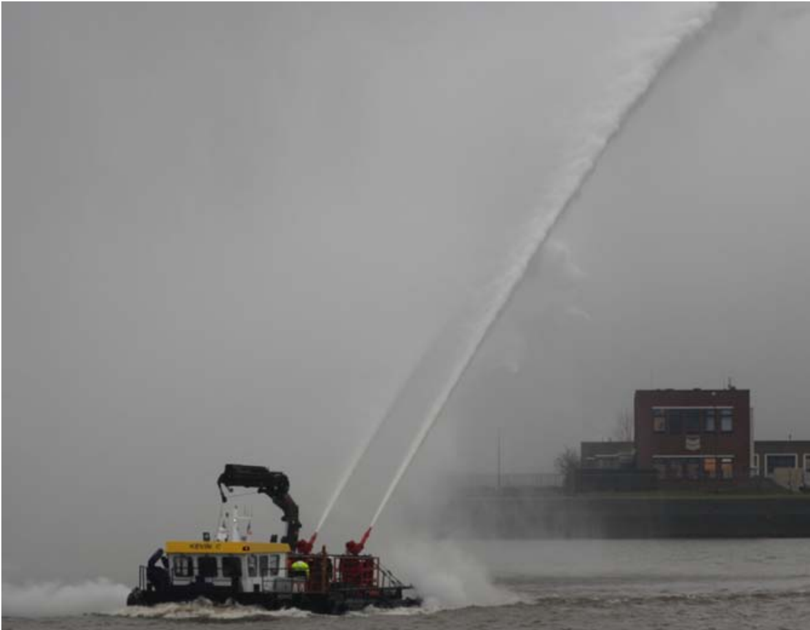
Seen on the Nieuwe Waterweg in Rotterdam the Kevin C , while MariFlex was testing 2 (portable) Fire Fighting units with a capacity of 12.000 l/min @ 12 bar.
