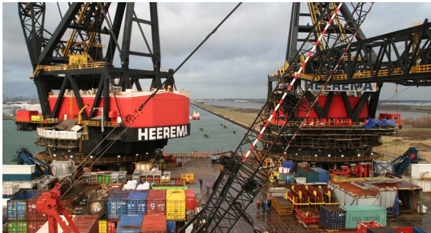
The workdeck of the THIALF with the two giant cranes - Photo : Lourens Visser ©
