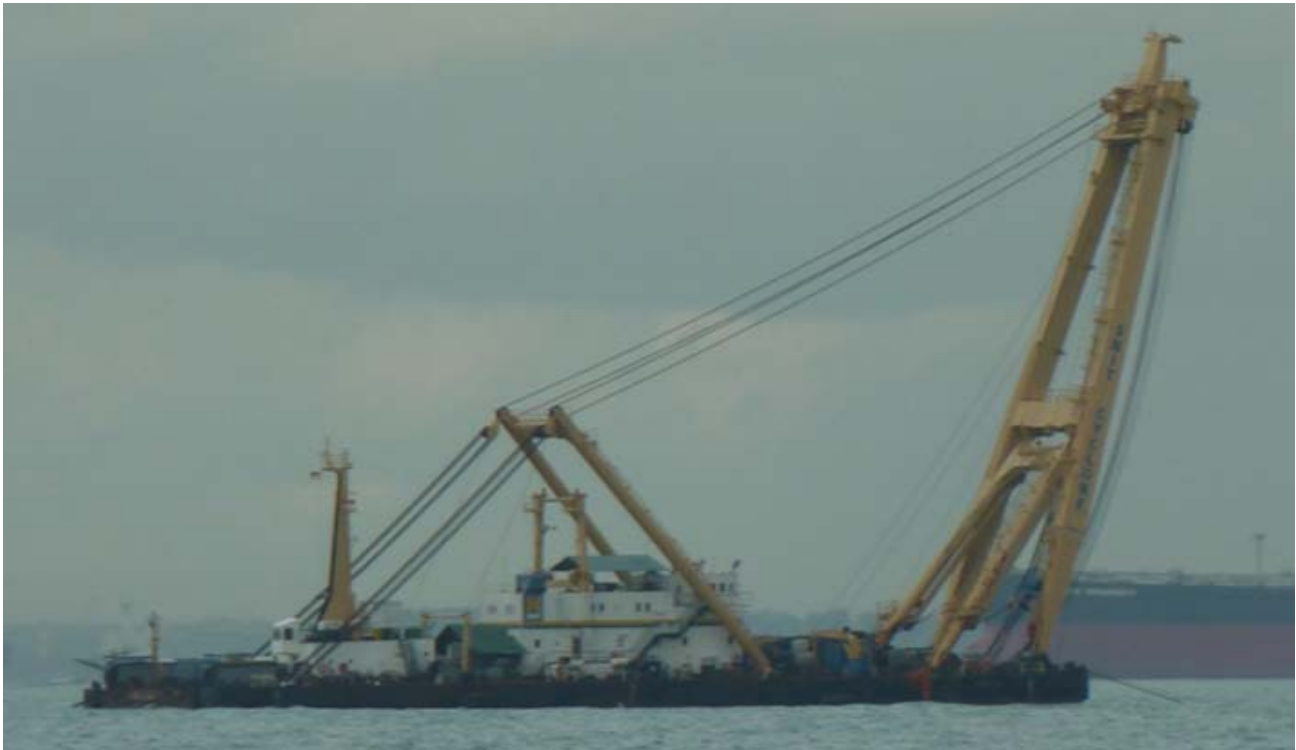
The Sheerlegs SMIT CYCLONE seen anchored over the wreck of the HYUNDAI 105 in the Singapore Straits
