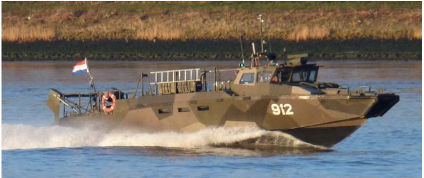
Another photo of the Swedish built Stridsbåt-90H-class 15.9 mtr long fast personnel landing craft [LCP] 912 which is serving the Royal Dutch Marines at present, above seen the craft enroute Rotterdam , the Aluminium built craft is able to carry a crew of 4 + 21 troops with a top speed of 40 knots - Photo : Frits Janse ©
