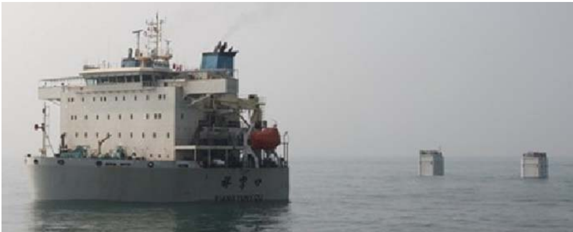
Above seen the new COSCO 50000 DWT Heavy Lift VESSEL during submerge trials off Hong Kong.
