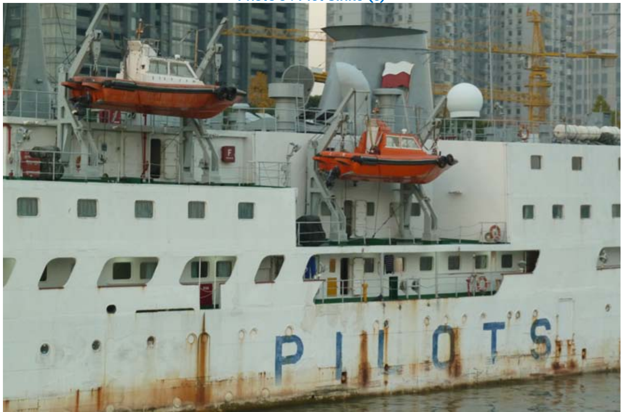
The Shanghai pilot cutter HUGANGYIN 1 seen moored "stand by" in Shanghai port, below seen the tenders onboard the cutter to transfer pilots from/to the mother ship to the arriving and departing ships
