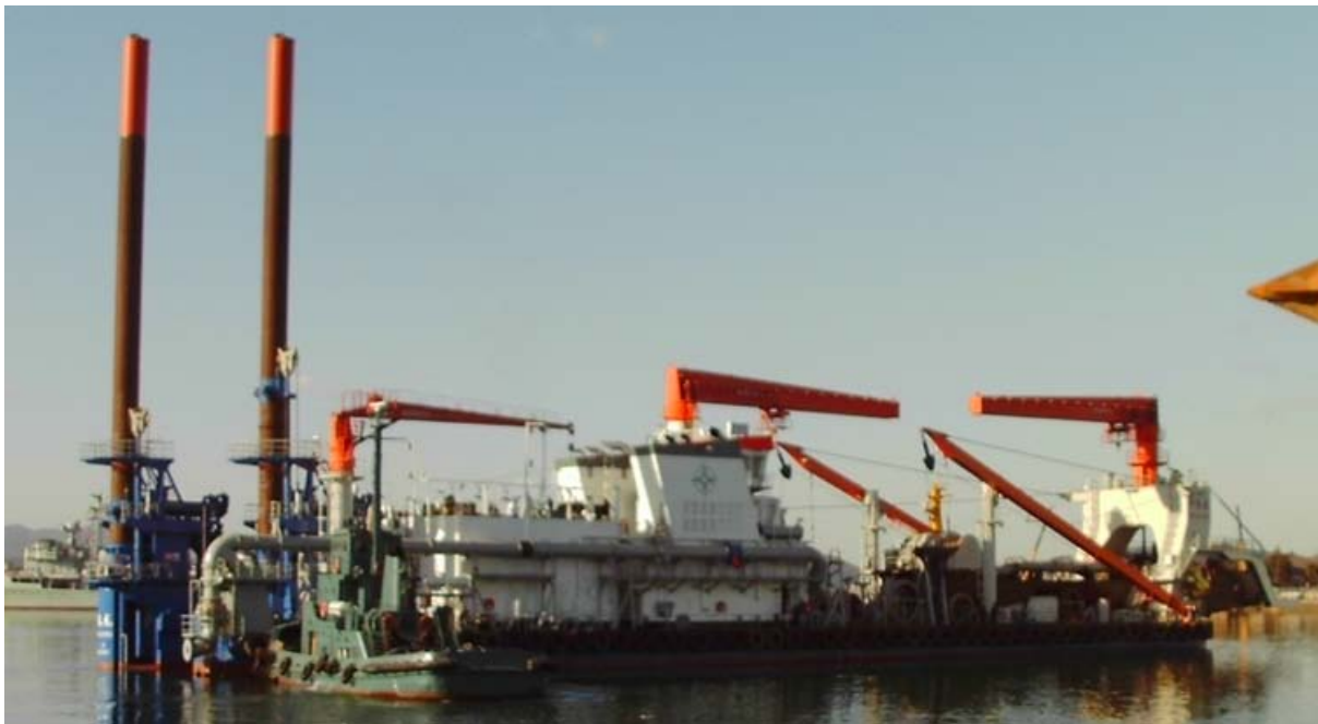
The first 8527 cutter dredger for GDC during trials at Dalian (China) build at DLS Dalian Shipyard for IHC Merwede . Dredging trials will be held in Rihzau Port in December.
