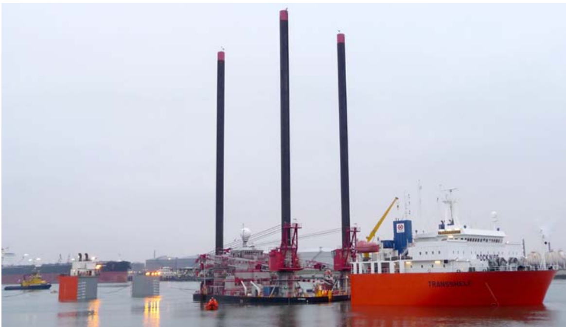
The TRANSSHELF seen loading the jack up KS TITAN 2 in Rotterdam-Caland canal
