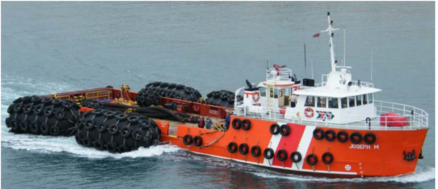
The 35.87m offshore supply vessel " Joseph M " of " A & J " company Ltd, Malta, ex "Mr Joseph". Built by Boconco Shipbuilding, Alabama, USA, in 1998, for Barry Graham Oil Sevices. Seen leaving Valletta with 4 fenders, for an offshore S.T.S operation. Photo : Gejtu Spiteri ©
