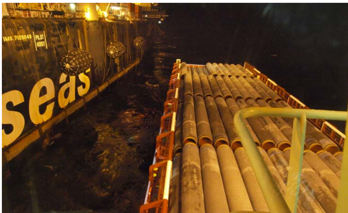
The Mærsk Fletcher seen with an almost full load of 112 pipes (totally 2,500 tons of cargo) alongside the Solitaire for discharging
