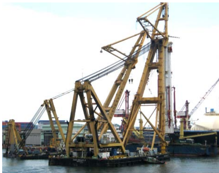
left seen the offloading by the 2 Asian Lift sheerlegs
