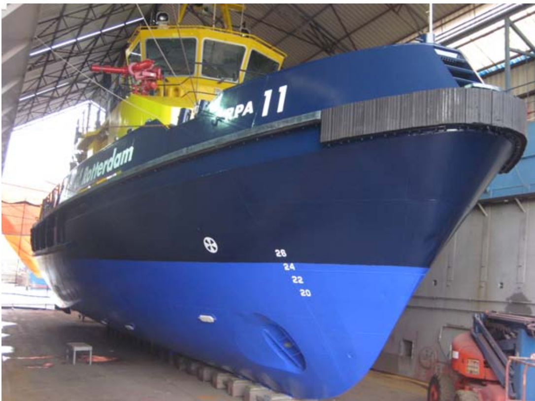
The RPA 11 (Port of Rotterdam) seen in Drydock at Maaskant Stellendam , after application of a new coat of paint, Intersleek®900, Fluoropolymer Foul Release Coating .
