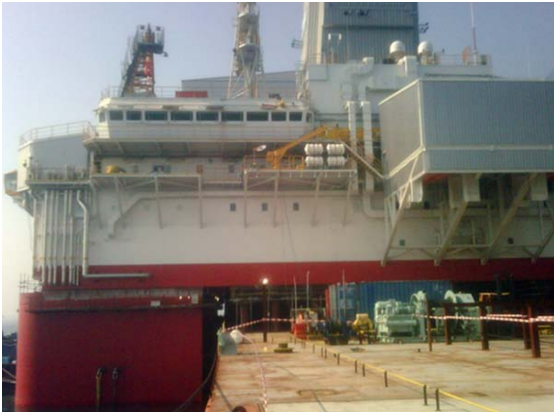
Above seen from the aft deck of the BLACK MARLIN while docked in between the the ballasted No. 2 Vyborg hull during the integration with No. 2 Vyborg topside .
