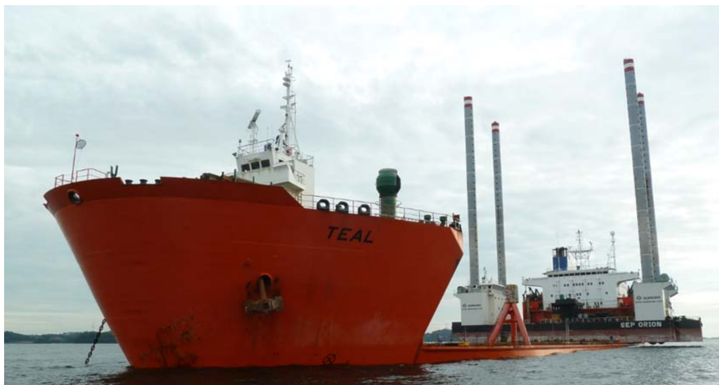
Dockwise TEAL seen submerging off Batu Ampar (Indonesia) to load the jack up rig SWIFT 10
