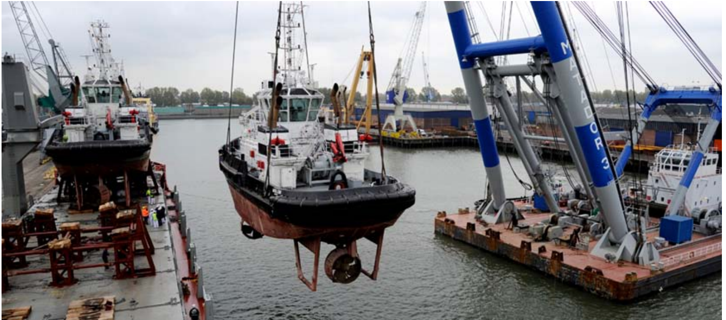
In the port of Rotterdam the sheerlegs MATADOR 3 offloaded the rotor tugs MIDLUM and DORUM , which arrived from Singapore onboard the CENA FAITH – Photo : Rob Niemandsverdriet ©
