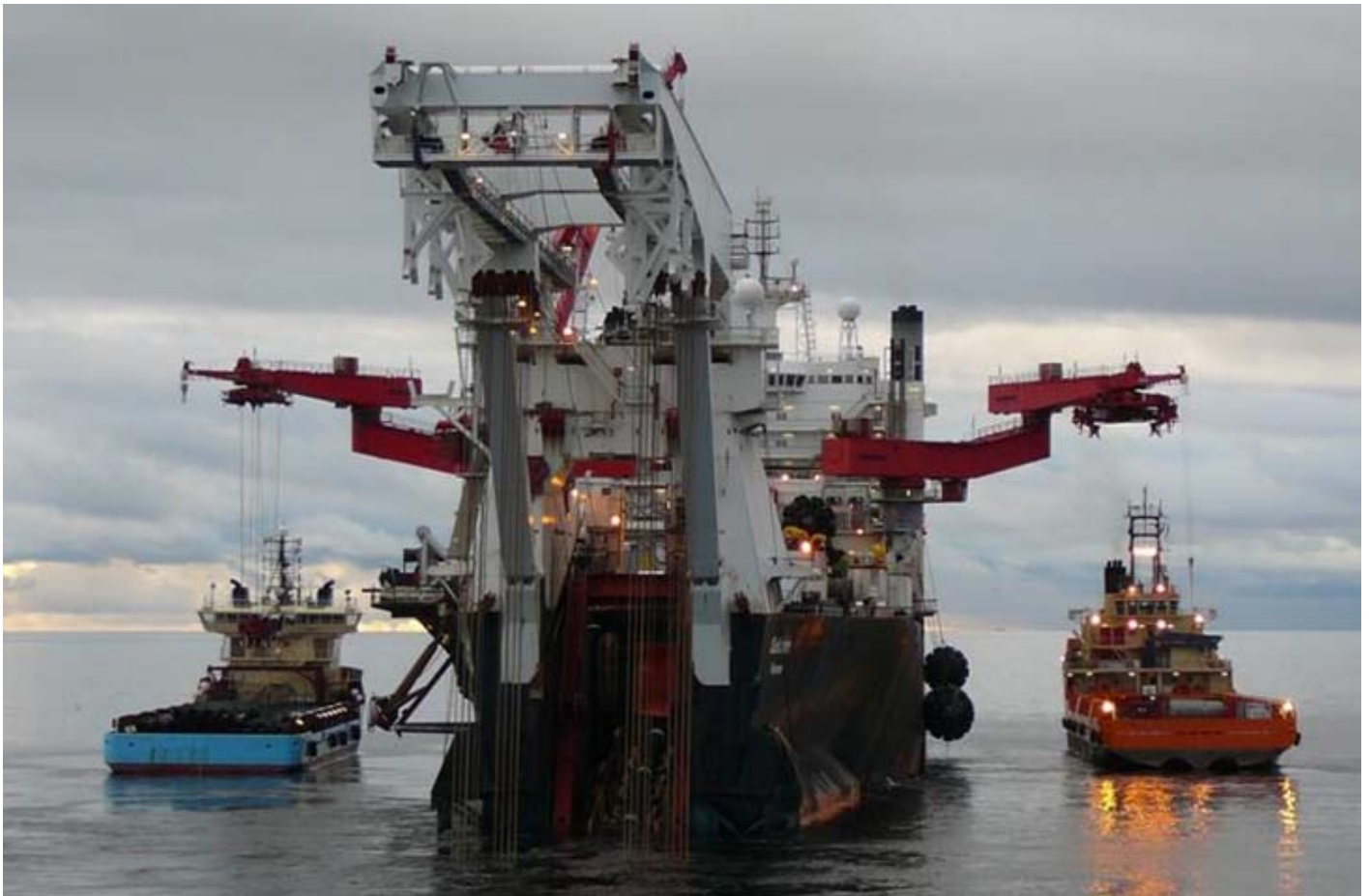
Above seen the Solitaire laying pipe on the Nord Stream natural gas pipeline with pipe carriers Maersk Fetcher and Toisa Independent working alongside. Photo is taken from the survey vessel Highland Rover .
