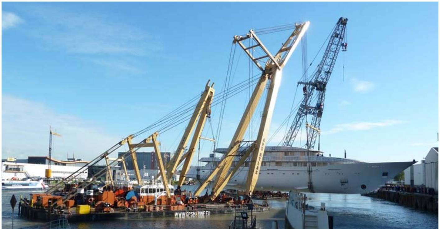
3 GPS shearlegs seen launching a newbuild luxury yacht at the Slob shipyard in Papendrecht (Netherlands)
