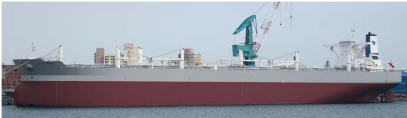
The E-WHALE (sister to the A-WHALE ) seen fitting out , she is the fifth ship out of a series of 5 built by Hyundai voor TMT, the tankers are 319869 DWT are 340m long and 60m width - Photo : Wouter van der Veen ©
