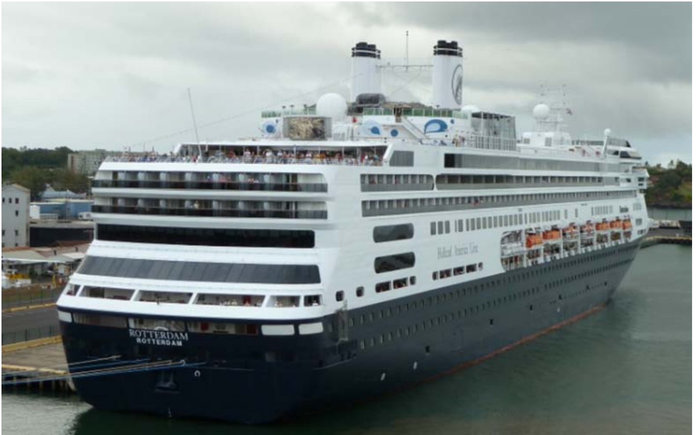
HAL' ROTTERDAM seen in her new look moored in Nawiliwili, in the back a whole deck was added to fire zone 1, approx 50 additional cabins, and a giant TV over the back deck
