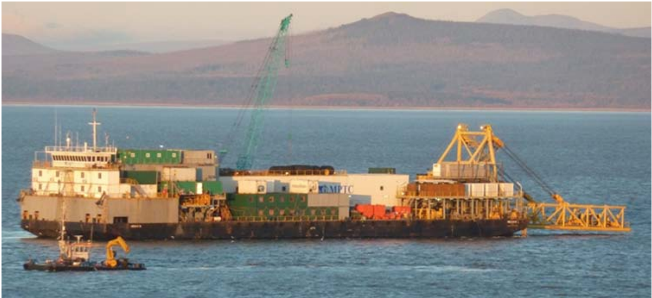
Above seen from the PLB Fortuna : MRTS PLB Nebula just completed the Sakhalin Gazprom 40" pipe line and in the process of recovering her anchors assisted by Multi Cat Nena W .
