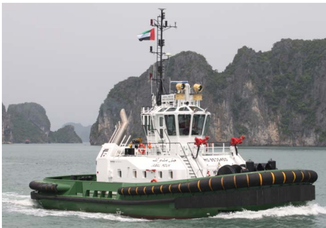
Above seen the ASD 2411 JABAL MDUK (68 ton Bollard Pull) during sea trials in Halong (Vietnam). The Jabal Mduk is build on Song Cam shipyards for Damen in Haiphong Vietnam under supervision of Damen surveyors under bnr 512236 for the port of Fujairah, This tug is the last of a series of three, Song Cam shipyard delivered earlier the Jabal Ghaf and Jabal Masafi also mentioned in news clippings number 174 . Photo : Ed Barten ©
