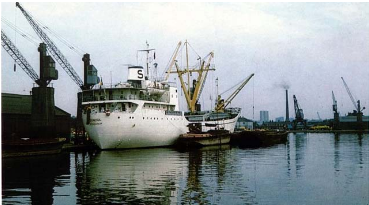
The 2400 ton GONDUL seen discharging cargo in London, the GONDUL was special designed to transport paper Photo : Coll. Kees van Huisstede ©
