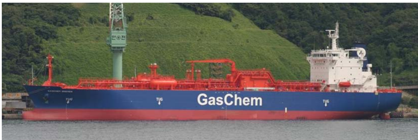
The GASCHEM BREMEN seen fitting out at the Hyundai yard in Ulsan, this vessel is the first out of a series of 3, the sisters will be named GASCHEM HAMBURG and GASCHEM STADE all with a capacity of 10.000 cbm
