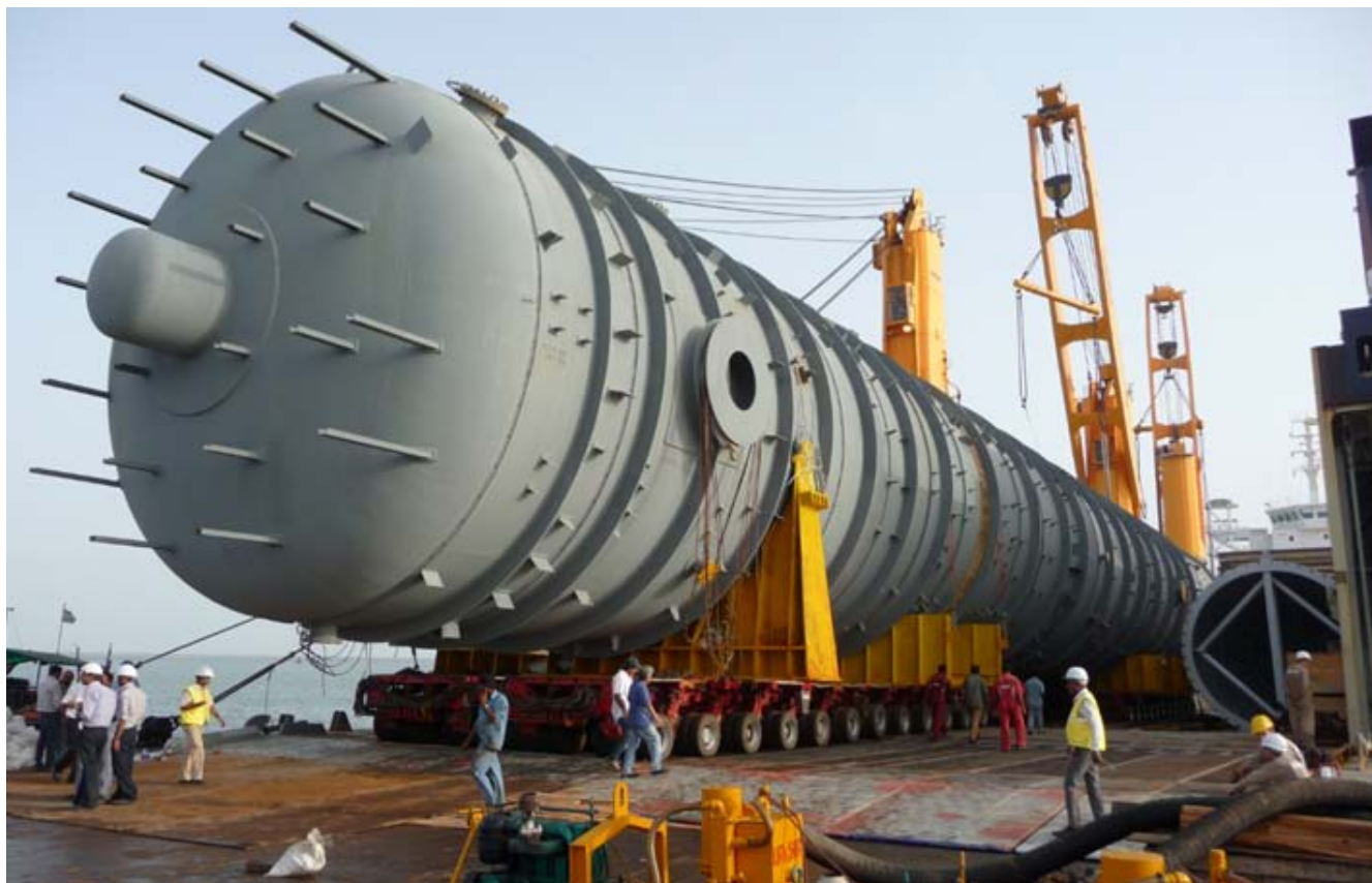
The COMBI DOCK I seen discharging a reactor onto a barge in India
