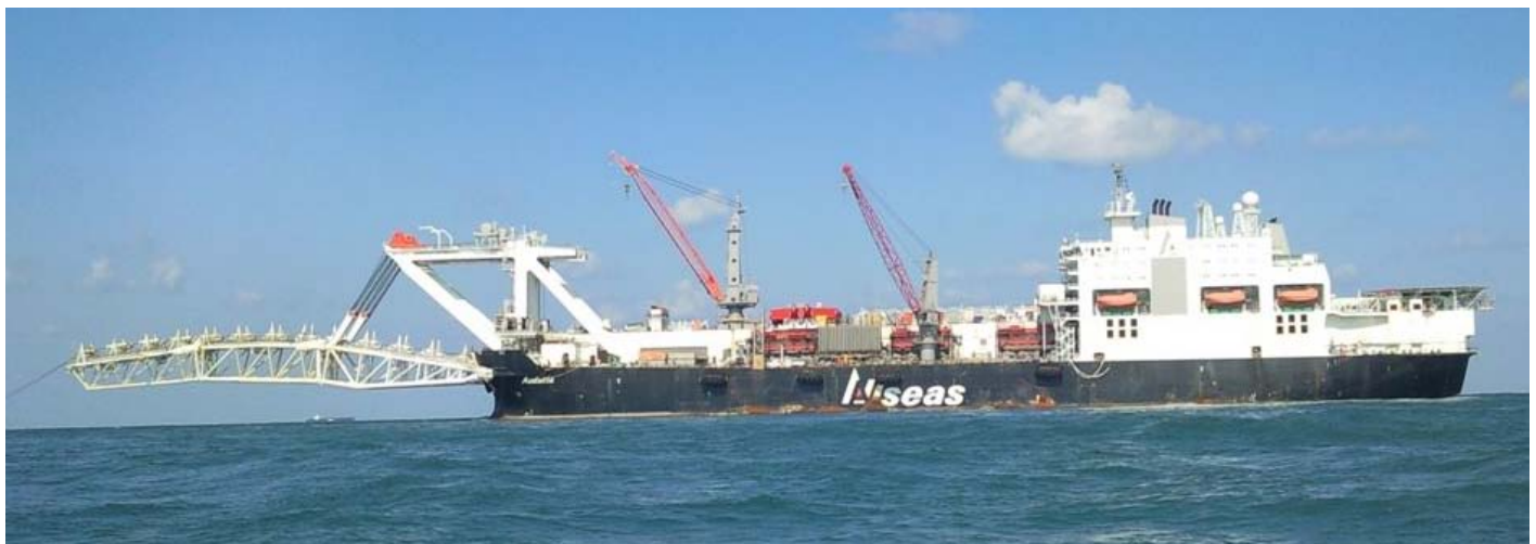
Allseas AUDACIA seen offshore Egypt working on the Burullus project where the pipelaying vessel is laying a 36" pipeline
