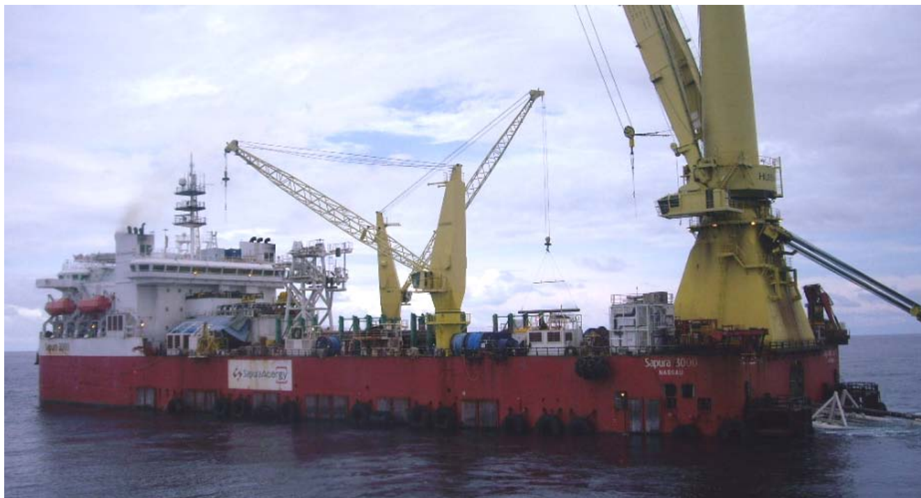
Above seen the SAPURA 3000 seen during pipelaying operation of an 24" pipe at the Gumusut project offshore Labuan (Malaysia), photo is made from the IDS CAHAYA which is the support vessel on this project
