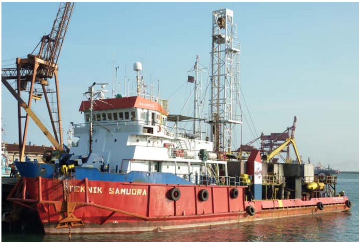
Still going strong, above seen the Patje Waterhuijzen 1975 built TEKNIK SAMUDRA (ex BROCO PEARL , ex. SMIT LLOYD 23 , ex SMIT MAASSLUIS ) moored in Kemamam supply base (Malaysia), this photo is special to me as editor, because myself sailed during 1992 > 1993 as captain on this vessel, the drilling capability within TEKNIK SAMUDRA allows for drilling up to 500 meters below seabed to investigate the absence of shallow gas, the vessel is owned and
